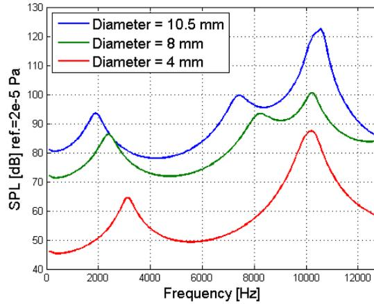
Fig. 10 – SPL results for the variation of the cavity and diaphragm diameter.
