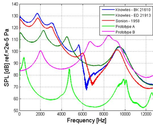
Fig. 11 – Comparison of Sound Pressure Level (SPL) of the commercial hearing aid loudspeakers and the piezoelectric loudspeaker prototypes ( $V = 1\text{Volt}$ ).
