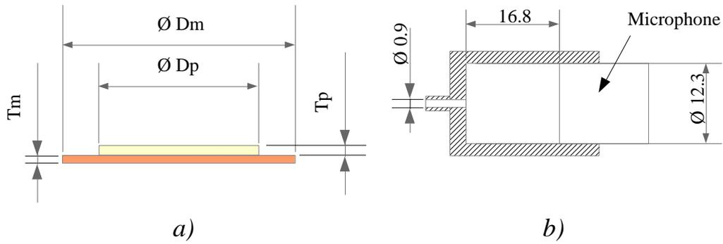
Fig. 2 – Dimensions (in millimeters) of the piezoelectric diaphragm (a) and the microphone coupler (b).
