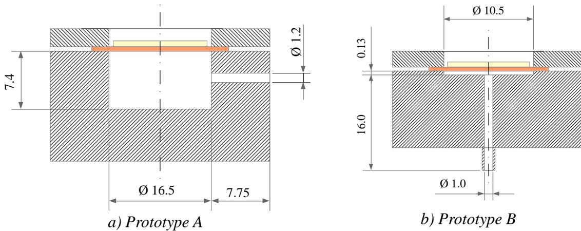
Fig. 3 – Dimensions (in millimeters) of the prototype loudspeaker cavities.
