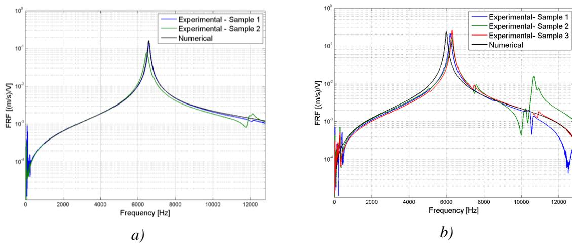
Fig. 6 – Comparison of numerical approach and experimental data for diaphragm A (a) and diaphragm B (b) in free mechanical boundary condition.
