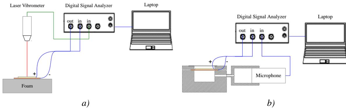
Fig. 4 – Experimental setups to take the measurement of the diaphragms in a free mechanical boundary condition (a) and it assembled with the loudspeaker cavities (b).
