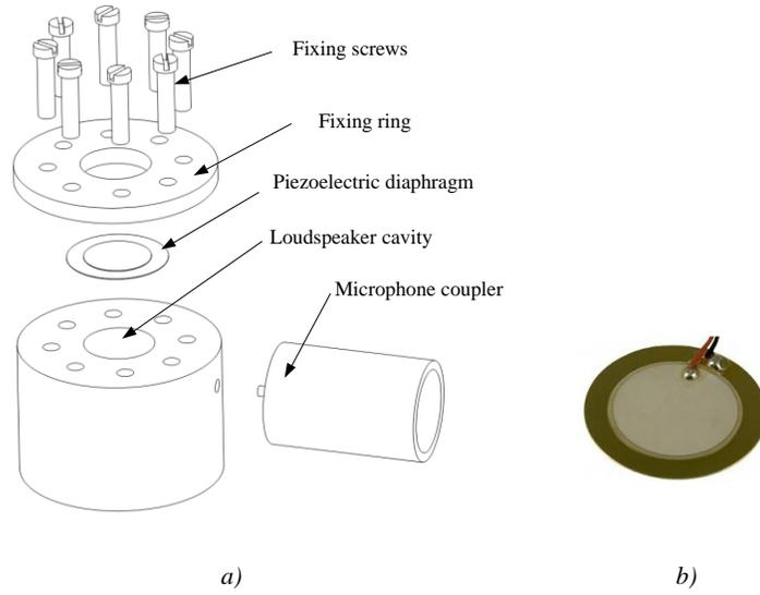
Fig. 1 – Components of the piezoelectric loudspeaker prototype with the microphone coupler (a) and a picture of the piezoelectric diaphragm used (b).
