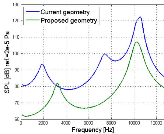
Fig. 12 – Comparison of the SPL for current Model B and a proposed geometry for a piezoelectric hearing aid loudspeaker ( $V = 1\text{Volt}$ ).
